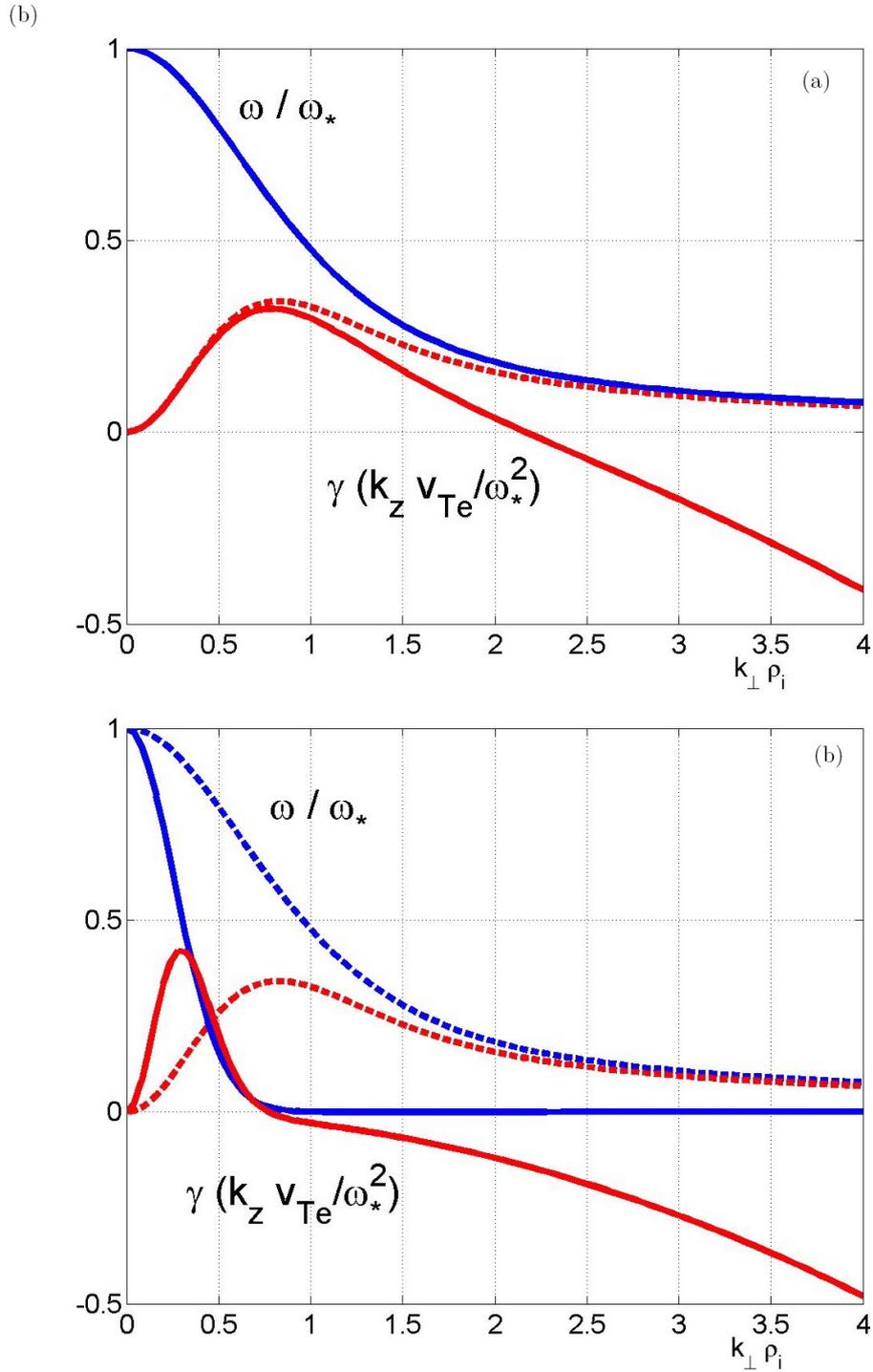
Figure 4: The wave number and the growth rate as function of the wave number for unperturbed plasma (dashed lines) and for turbulent plasma (continuous lines). The Kubo number of the background turbulence is  $K = 0.1$  in (a) and  $K = 10$  in (b).
