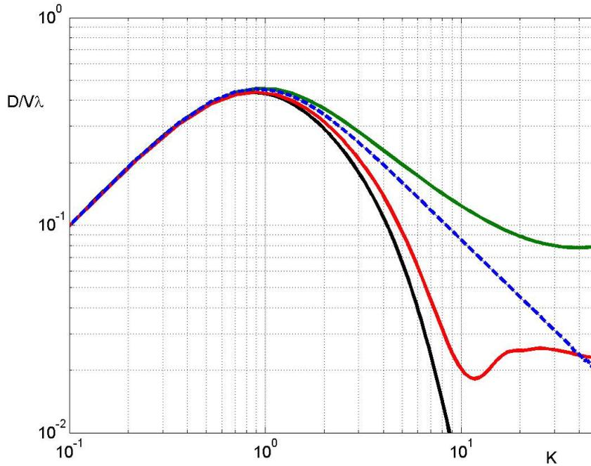
Figure 2: The diffusion coefficient as function of  $K$  for the values of  $V_p/V$ ,  $\chi/V\lambda_c$ : 0, 0 (blue); 0.4, 0 (black); 0, 0.02 (green); 0.4, 0.02 (red).
