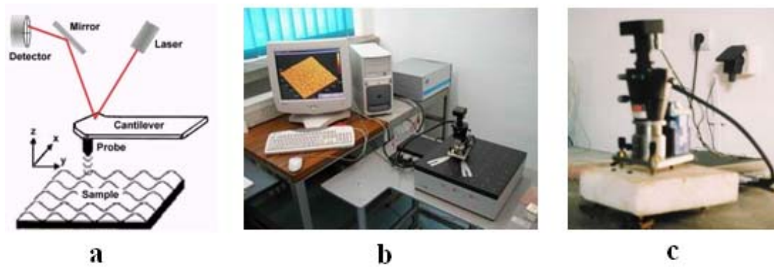
Figure 4: Schematic of the atomic force microscope principle (a) and actual images of the microscope setup (b and c).
