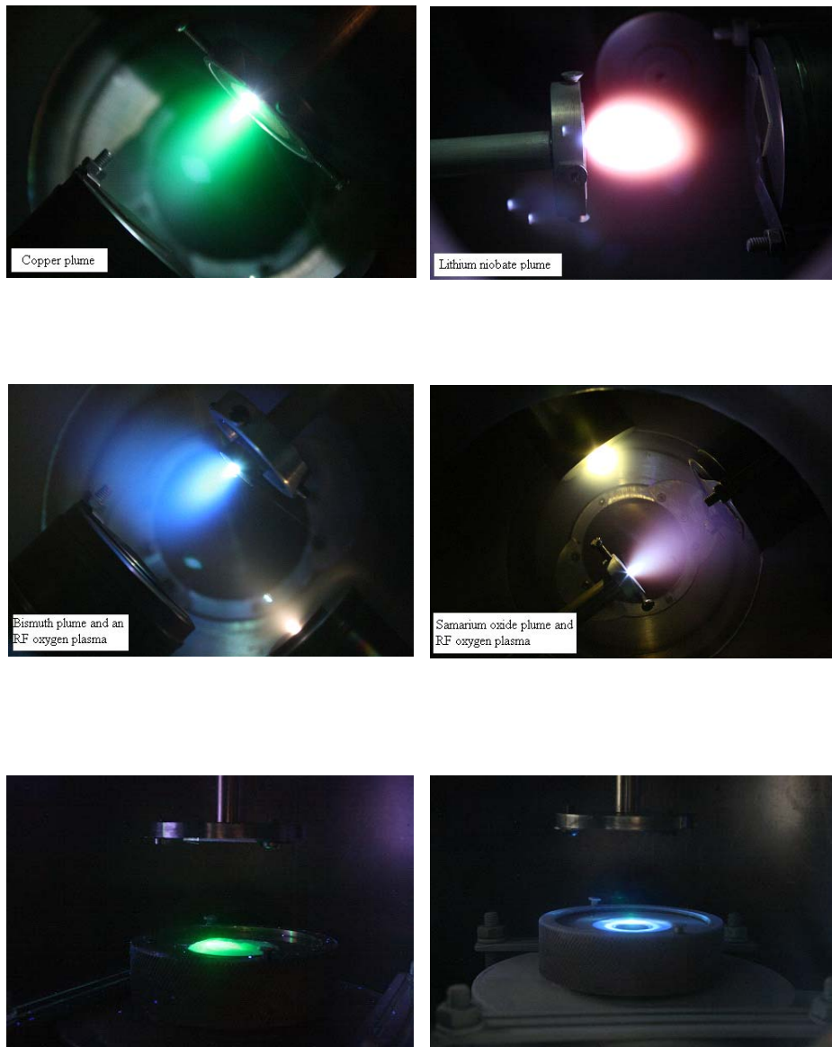
Figure 7: Examples of plasma plumes produced during PLD (a), RF-PLD (b) and MAPLE (c) procedures.
