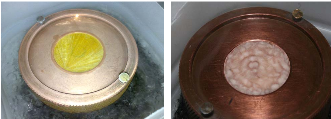
Figure 4: Photographs of a MAPLE target holder during the cryogenic procedure (in liquid nitrogen, 77K): freezing a solution of \text{Cu}(\text{DAB})_2 , a complex metal-organic hybrid compound, dissolved in toluene (a) and while freezing a solution of lactoferrin (a protein) dissolved in deionized water (b).
