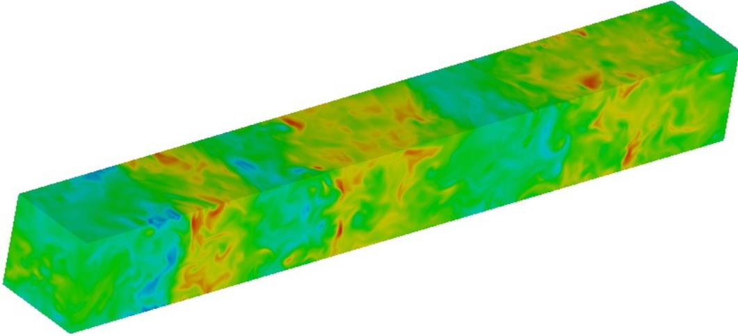
Figure 1: Turbulence intensities in the Kolmogorov flow. The largest size of the box corresponds to the  $x$  (streamwise) direction. This figure clearly shows that the translational invariance in the streamwise direction is broken.
