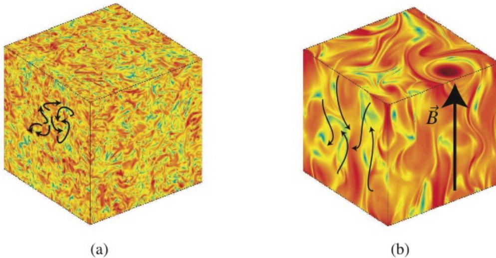
Figure 3: The left figure represents energy density contours for an initial isotropic turbulent velocity field in a conducting fluid. The right figure represents the same quantity for the anisotropic state predicted by the QSA. The magnetic field is directed in the vertical direction.
