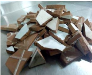
Figure (2) Crushed ceramic after washing and drying
