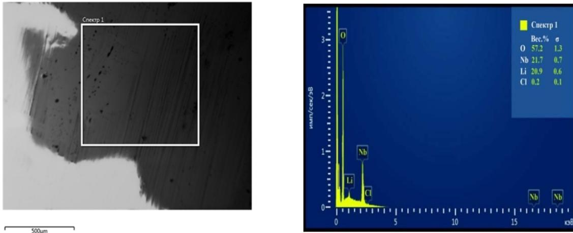
**Fig. 1.** SEM image of a pure lithium niobate crystal and elemental analysis results
