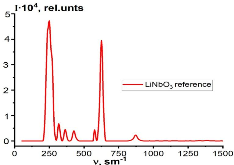
Fig. 5. Raman spectra of lithium niobate
