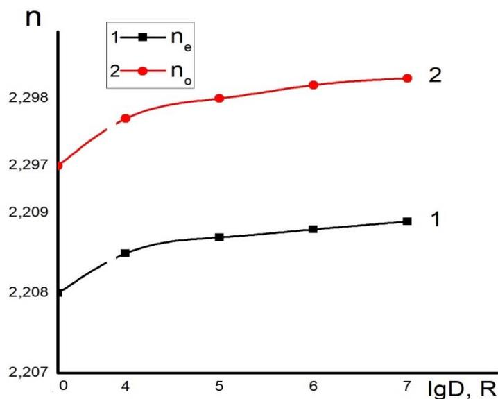
**Fig. 3.** Dependences of  $n_e$  and  $n_o$  on the dose of  $\gamma$ -radiation for LiNbO<sub>3</sub> crystals
