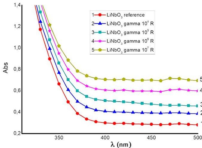
**Fig. 2.** Absorption spectrum of irradiated and non-irradiated  $\text{LiNbO}_3$
