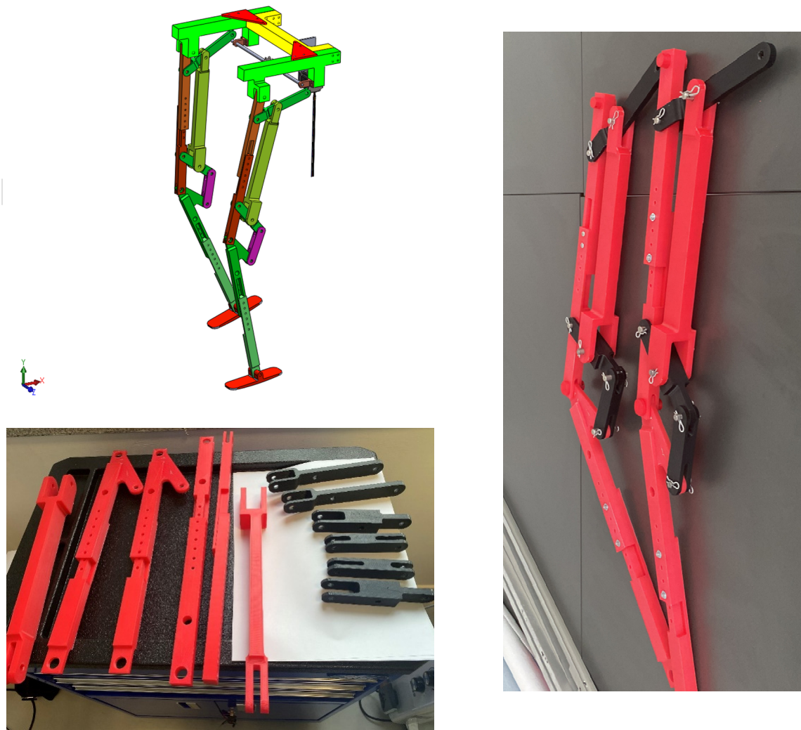
Figure 16. Exoskeleton components made by 3D printing for assembly purpose
