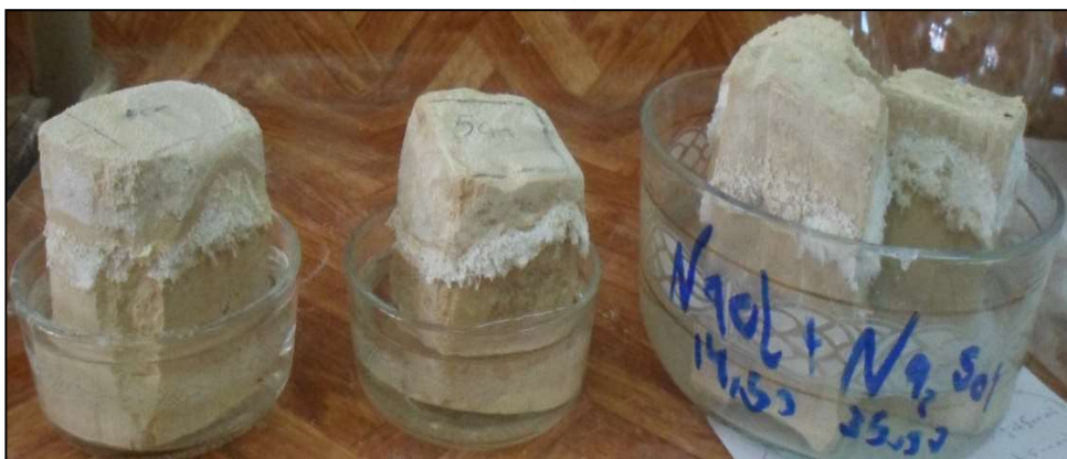
Fig.5. Illustrates efflorescence of salts over blocks in the presence of water
