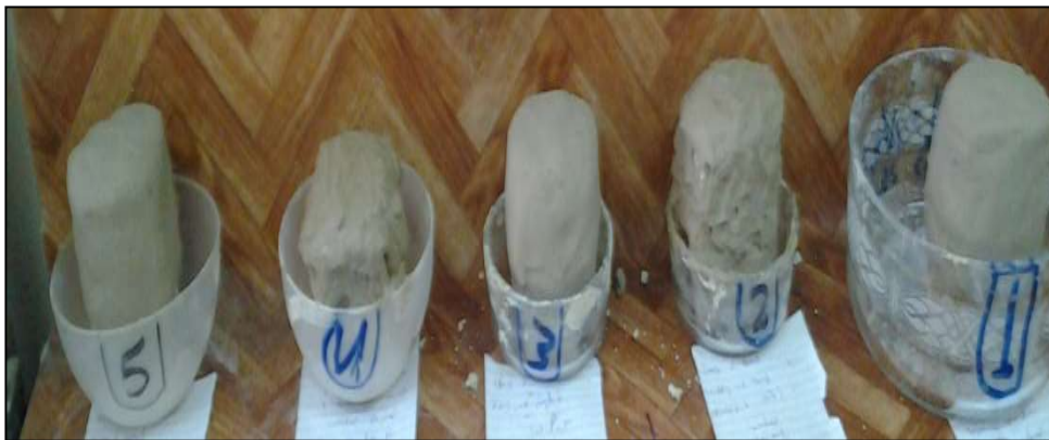
Fig.6. Illustrates the application of different wet bentonite poultices
