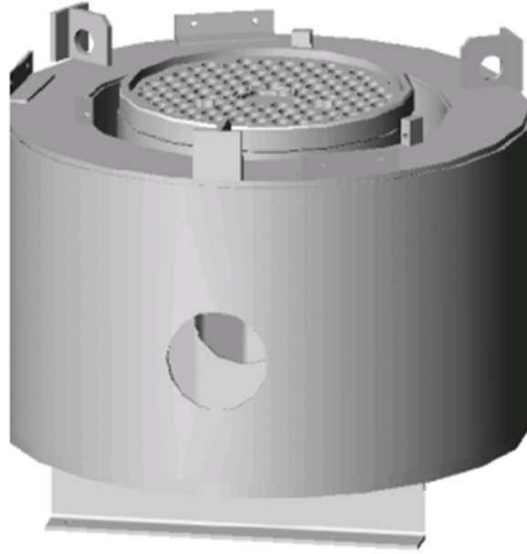
Figure 2. The reflector assembly of the TM2 reactor.
