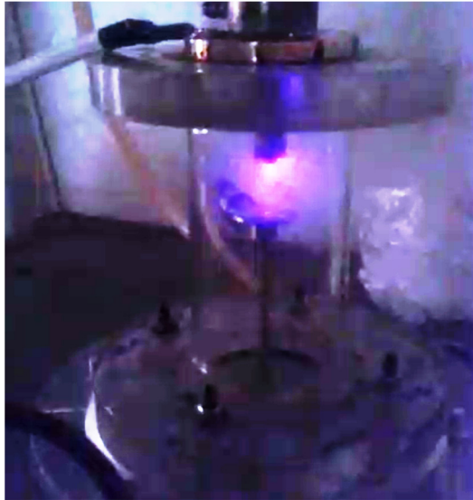
Figure 2: The photograph of light emission from pulsed DC hollow cathode plasma jet
