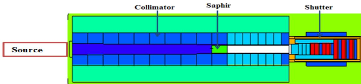
Figure 2. 2D models of collimator and shutter, obtained by the code MCNP
