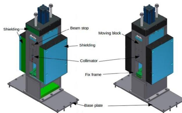
Figure 1. Neutron Beam Shutter for PGAA
