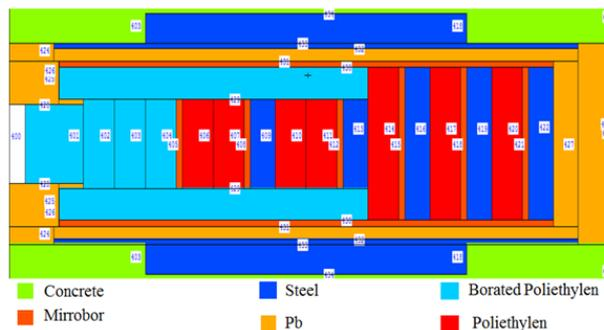
Figure 3. 2D model of the shutter, obtained by the code MCNP
