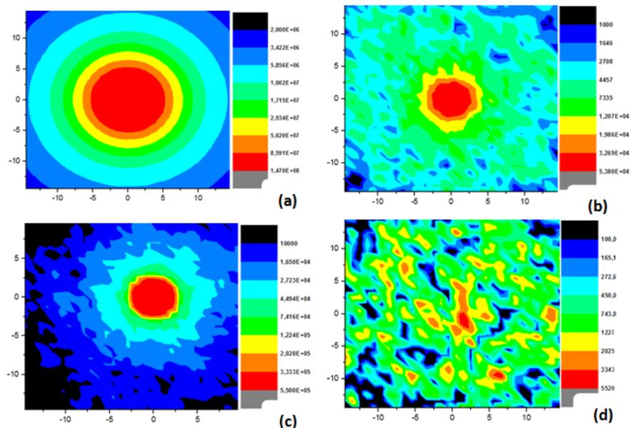
Figure 6. Neutron flux mapping was carried out at 10 cm from the collimator inlet (a), at the end of the collimator (b), at 20 cm from the shutter inlet (c) and 40 cm from the shutter inlet (d)
