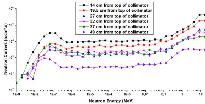
Figure 5. Neutron flux distribution in different shutter position
