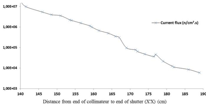
Figure 4. Neutron flux distribution through shutter (n/cm<sup>2</sup>.s)
