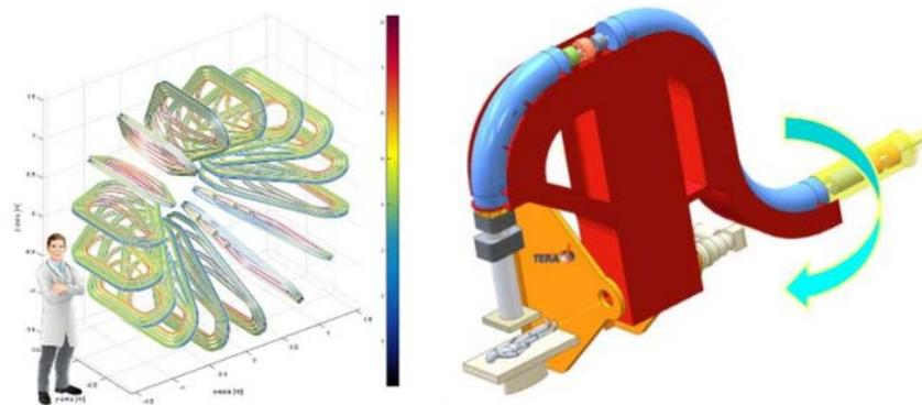
**Figure 6.** (left): schematic of the coils of the Ga-Toroid (the beam would pass in between the coils) (source CERN), (right): schematics of the compact 1800 rotating gantry (source TERA Foundation).
