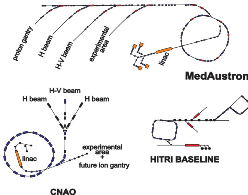
**Figure 5.** Overall size of the SEEIIST (HITRI) footprint compared to CNAO and MedAustron ion treatment facilities. HITRI baseline based on superconducting synchrotron - drastic reduction in the footprint (area).
