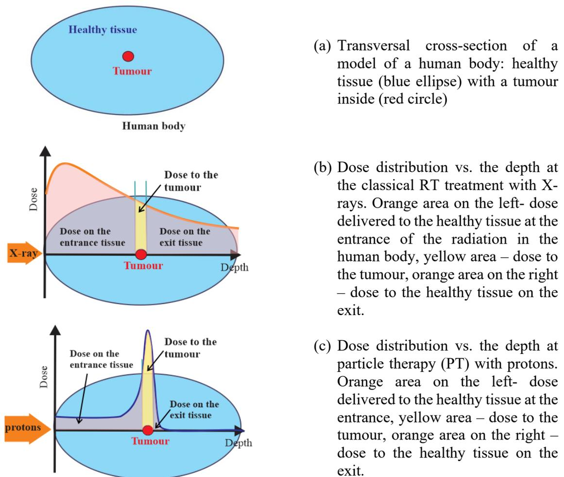
**Figure 3.** Comparison between the dose distribution in the targeted tumour and the healthy tissue in a model of a human body.
